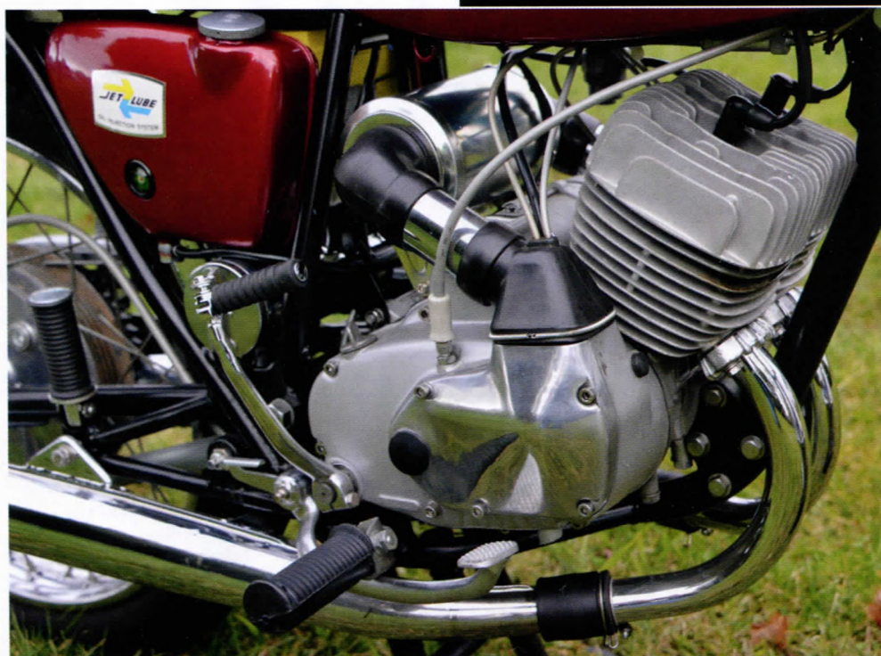
BELOW Right side of the bike, with the generator visible under the cylindrical air filter that sits neatly behind the engine.
