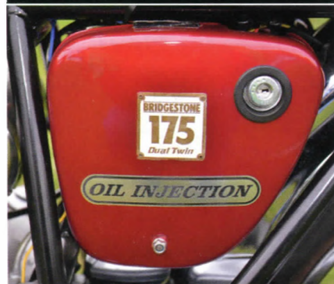
ABOVE CENTRE Oil tank with tool box underneath. ABOVE Oil pump sits behind left cover, with the black line running to the tank on the opposite side. Lever above the rocking pedal is to shift the gear selection from four to five speed.
