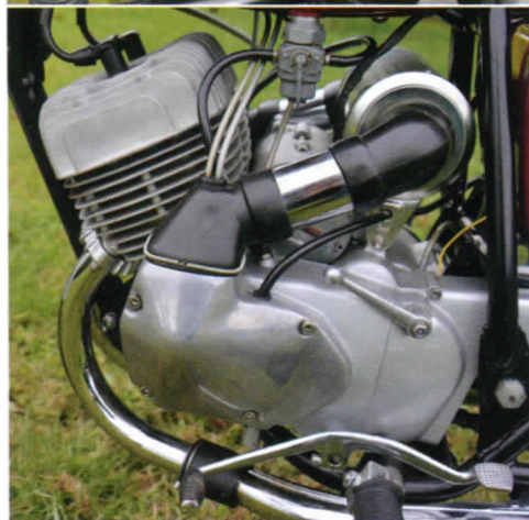
ABOVE CENTRE Oil tank with tool box underneath. ABOVE Oil pump sits behind left cover, with the black line running to the tank on the opposite side. Lever above the rocking pedal is to shift the gear selection from four to five speed.
